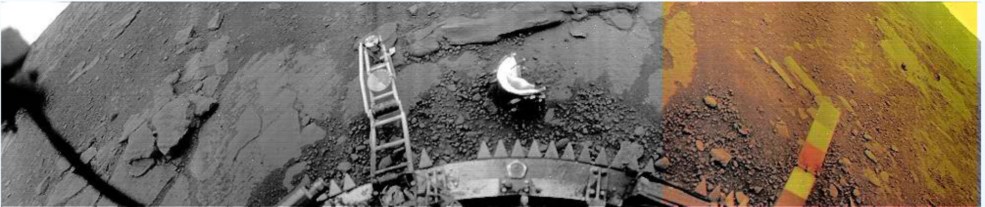
Venera 13, camera 1, spring loaded soil sampler
