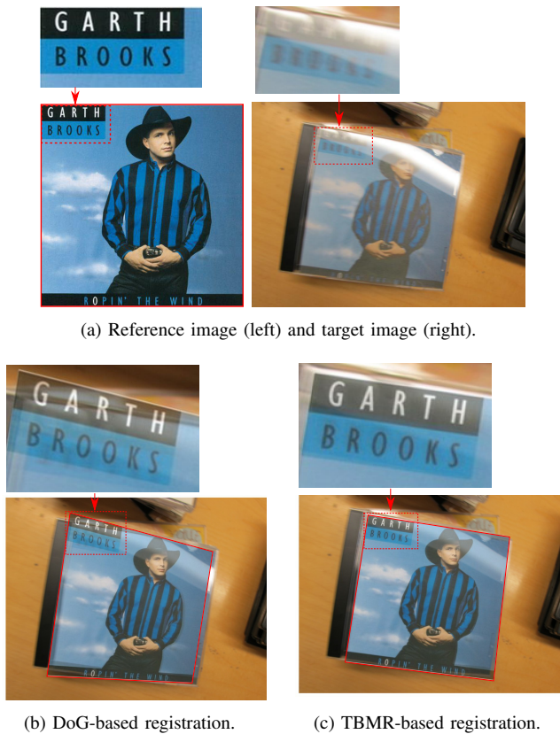
Fig. 11. Homographic registration of a pair of images. The result obtained using DoG (b) is not as accurate as the one based on TBMR (c); see the zoomed top left corner. Harris-Affine, Hessian-Affine, and MSER all fail in registering this pair of images.
